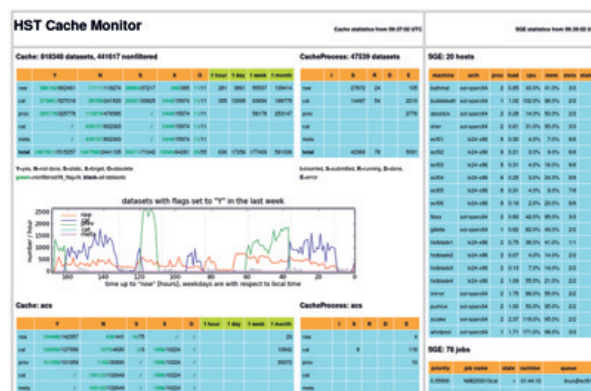
Fig 1: HST Cache monitor. A web interface to continuously updating statistics on the progress of Cache processing.
